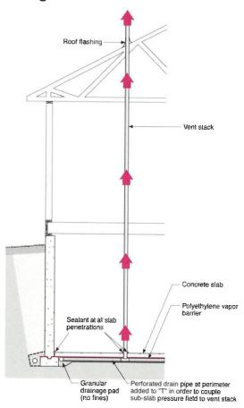
A passive sub-slab depressurization system shall be installed during construction in basement or slab-on-grade buildings.
