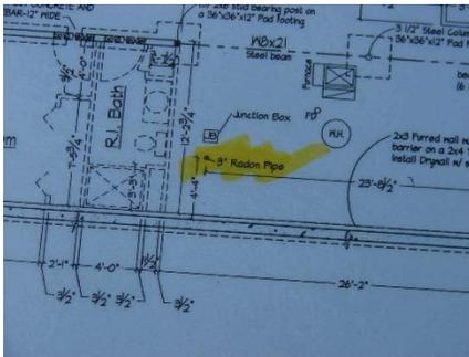
←A PSGVS is a formal building system. As such, it should appear on the construction drawings for all floors. When the passive SGVS appears on the set of construction blueprints, almost any worker can ensure that it is installed properly in the intended location
